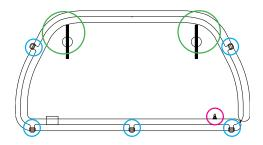
Fasten inflated screen with included fasteners. Fasteners are adjustable in lenght using the robe stopper. Find the proper position to fixate the shield, such that it is nicely tensioned.
